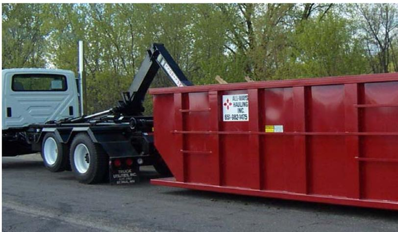
The Ampliroll Hook Lift was invented in 1969. Our process of laser cutting and robotic welding enables us to provide you with a complete line of hooklifts, that eliminate the use of **SHIMS** and **WEAR PADS**.
